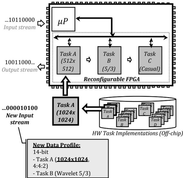
Figure 1: Reconfigurable computing relies on splitting an application into many different tasks. These tasks are then written in hardware and can be loaded onto the chip depending on parameters in a hardware data profile. Image from [13].
