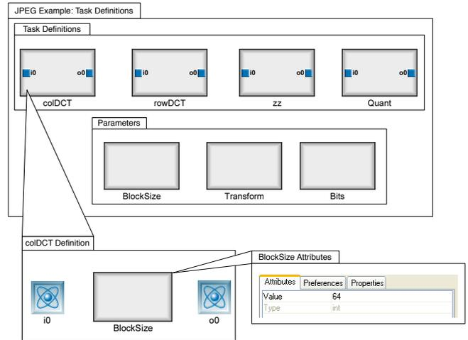
Figure 4: The JPEG example has three main parameters: *BlockSize*, *Transform*, and *Bits*. Those parameters and their values define which hardware configuration will be used for any given data stream. The inside of a configuration of the *colDCT* task is also shown in the figure. This shows that the *BlockSize* parameter is the only parameter that defines that task. It also shows that the *BlockSize* parameter has attributes for its value and that value's type.
