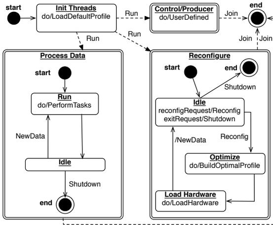
Figure 5: The state-chart diagram of the Overseer Methodology. This figure shows that the basic concept is to have a user defined control thread, a generated reconfiguration thread, and the task threads (shown here as one ‘process’ thread for simplicity). These three threads are spawned by an initialization process then the application completes when all three threads complete.
