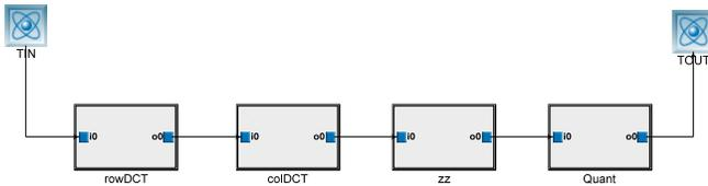
Figure 3: Model of the streaming JPEG example application. It consists of four application tasks plus a terminal producer and terminal consumer.
