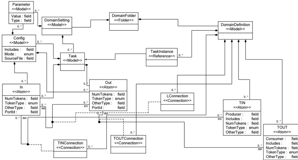
Figure 2: The metamodel for DaresML defines how users can model DARES projects. This model has been updated from [6], though the core components have not changed.
