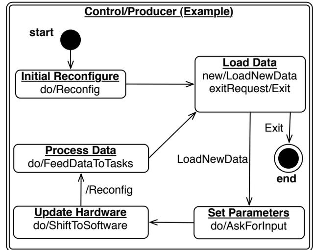
Figure 6: This is an example of how a user defined control thread might act. DaresML provides the user with the semantic structures to set parameters, update the hardware, and the initial reconfiguration. The user is responsible for loading the data stream. Note that the *Reconfig* method refers to Fig. 5.
